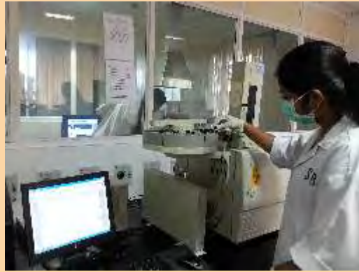
GC with ECD Disulfoton etc are analysed by Gas Chromatograph with FPD.(Flame Photometric Detector)
